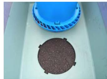
Insert the StormBasin cartridge down through the hole in the base of the unit. The colored ring on the cartridge should be facing upwards. Push the cartridge all the way through the hole until it rests on the bottom. Slowly turn the cartridge in a Clock-wise direction until the Tabs align with the slots and the cartridge body drops about  $\frac{1}{4}$ ' further down.
