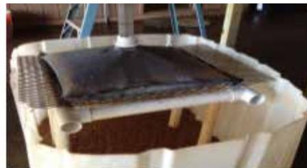
The results from this test prove the fact that the ACF Dirtbag® becomes more efficient once a sediment coating builds up on the inside walls of the Dirtbag®, while producing discharged water that is visibly clear due to the smaller particles being retained by the sediment coating.
